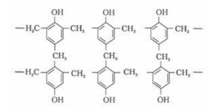
It is used for making combs, phonograph records, electrical switches and handles of various utensils
