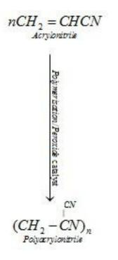
It is used as a substitute for wool in making commercial fibres such as orlon or acrilan.
