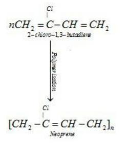
It is used for manufacturing conveyor belts, gaskets and hoses
