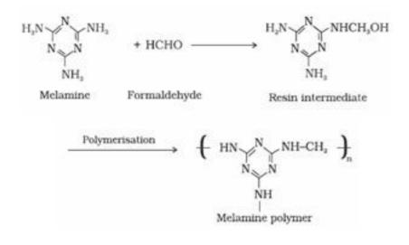
It is used in the manufacture of unbreakable crockery.
