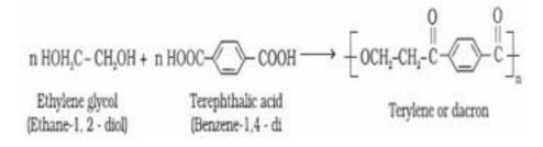
It is used to create resistance in polymerised product and is used in blending with cotton and wool fibres and also as glass reinforcing materials in safety helmets, etc.
