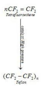
It is used in making oil seals and gaskets and also used for non – stick surface coated utensils
