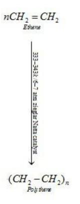
It is used for manufacturing buckets, dustbins, bottles, pipes, etc.
