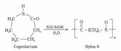
It is used for the manufacture of tyre cords, fabrics and ropes.
