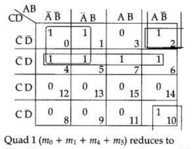
Quad 1  $(m_0 + m_1 + m_4 + m_5)$  reduces to Quad 2  $(m_4 + m_5 + m_6 + m_7)$  reduces to D Pair 1  $(m_2 + m_0)$  reduces to A Hence, F(C, D, A, B) = + D + A
