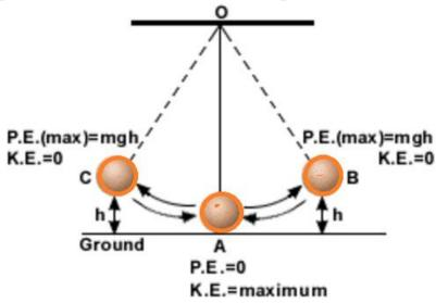
At the points B and C, the pendulum bob is at its maximum height, so its potential energy is maximum and kinetic energy is zero. In this way the total mechanical energy remains constant. At the point A, the pendulum bob is at its lowest point, total potential energy is converted into kinetic energy. Now the kinetic energy is maximum and potential energy is zero. Once again the total mechanical energy remains constant.
