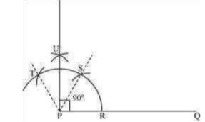
We have,  $\angle$  SPQ =  $\angle$  TPS = 60°. In (iii) and (iv) steps of this construction, PU was drawn as the bisector of  $\angle$  TPS.
