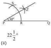
The below given steps will be followed to construct an angle of  $22\overline{2}^{\circ}$ .
