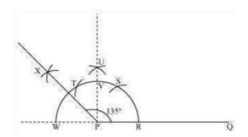
The angle so formed can be measured with the help of a protractor. It comes to be 135°.
