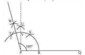
The angle so formed can be measured with the help of a protractor. It comes to be 105°.
