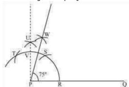
The angle so formed can be measured with the help of a protractor. It comes to be  $75^{\circ}$ .
