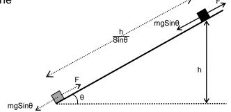
Min force required to push the body is  $F = mgSin\theta$ And displacement of body in lifting is  $s = \frac{h}{Sin\theta}$ Hence work done in pushing is or,  $W_2 = FsCos0$   $W_2 = mgSin\theta \cdot \frac{h}{Sin\theta} \cdot 1$ or,  $W_2 = mgSin\theta \cdot \frac{h}{Sin\theta} \cdot 1$
