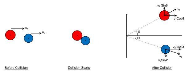
When the centers of mass of two bodies are not along the same straight line, the collision is said to be oblique. In such condition after collision bodies are deflected at some angle with the initial direction. In this type of collision momentum conservation is applied separately along x-axis and y-axis. If the collision is perfectly elastic energy conservation is also applied.
