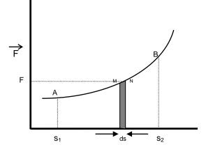
To find work done from  $s_1$  to  $s_2$  we consider two points M & N very close on the graph such that magnitude of force (F) is almost same at both the points. If elementary displacement from M to N is ds, then elementary work done from M to N is.
