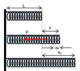
Consider a spring of natural length 'L' & spring constant 'k' its length is increased by  $x_0$ . Elastic potential energy of stretched spring will be equal to total work done by the spring in regaining its original length.
