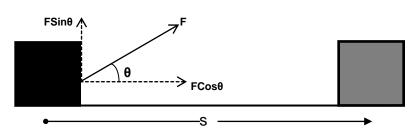
If force and displacement are not parallel to each other rather they are inclined at an angle, then in the evaluation of work component of force (F) in the direction of displacement (s) will be considered.
