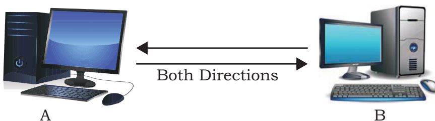
Figure 11.5: Full duplex transmission of data
