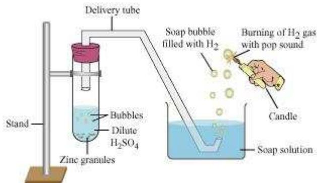
Take few pieces of zinc granules and add 5 ml of dilute H<sub>2</sub>SO<sub>4</sub>. Shake it and pass the gas produced into a soap solution. The bubbles of the soap solution are formed. These soap bubbles contain hydrogen gas.
