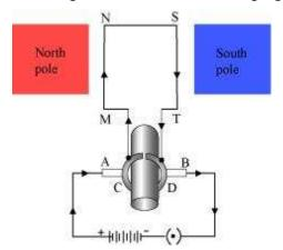
When a current is allowed to flow through the coil MNST by closing the switch, the coil starts rotating anti-clockwise. This happens because a downward force acts on length MN
