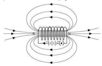
In the above figure, when the north pole of a bar magnet is brought near the end connected to the negative terminal of the battery, the solenoid repels the bar magnet. Since like poles repel each other, the end connected to the negative terminal of the battery behaves as the north pole of the solenoid and the other end behaves as a south pole. Hence, one end of the solenoid behaves as a north pole and the other end behaves as a south pole.
